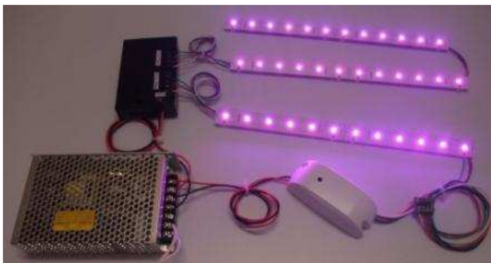
<AWCL-120-6P connects with the Signal repeater by lightings>
